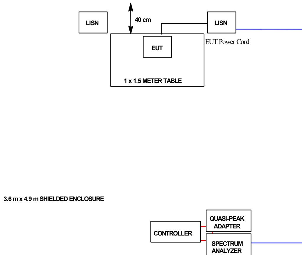
**FIGURE 2: Radiated Emissions Test Setup**
