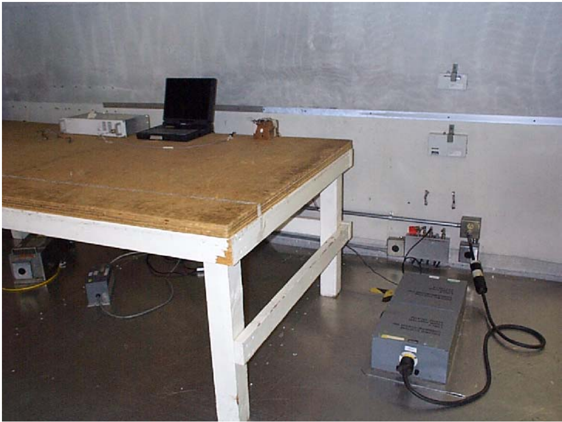
Photo 2 – Line Conducted Emission Testing
