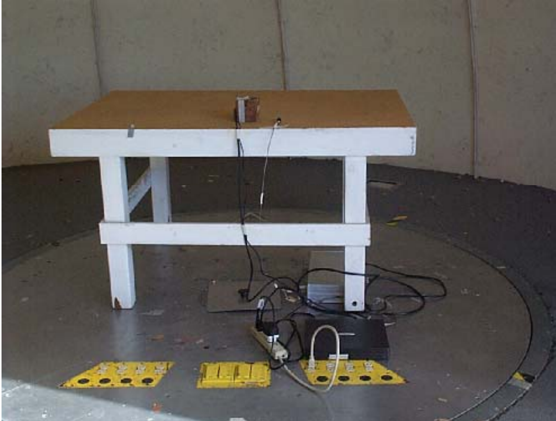
Photo 1 – Radiated Emission Testing at Open Area Test Site
