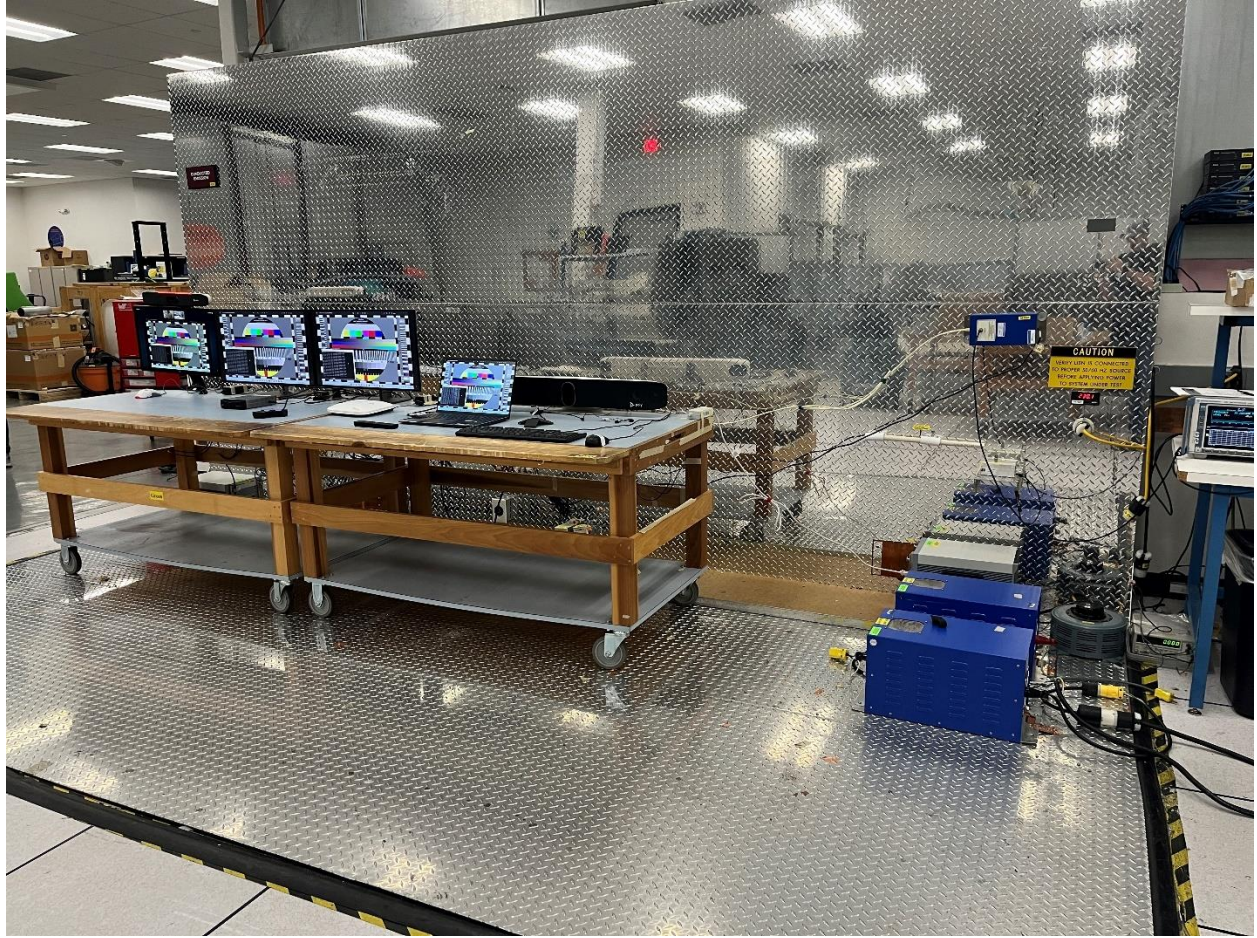
Conducted Emissions Overall Setup
