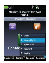
2 Press the 2 key or scroll to 2 Keypad Lock, and press OK. Once you lock the keypad, all the keys become frozen except for an Unlock soft key, which replaces the Features soft key.
