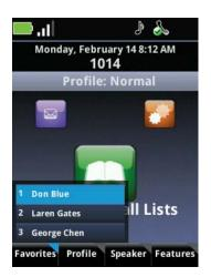
You can select one of these names or use the keypad to press a speed-dial index number. The call is placed immediately. See *Enabling and Disabling DND on all lines when single line DND is enabled*.
