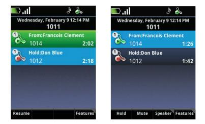
An active call has a light blue field when it is highlighted. An active call has a green field when another session cell is highlighted. Soft key presses affect highlighted cells. In the above example, you can see how the soft keys change when you highlight an active call.
