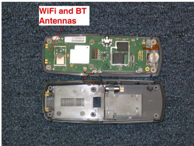
PCB with Antenna Locations
