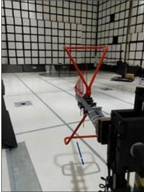
Photograph 1. Radiated Spurious Emissions, Below 1 GHz, Test Setup
