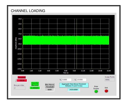
The level of traffic loading on the channel by the EUT is 24.19%
