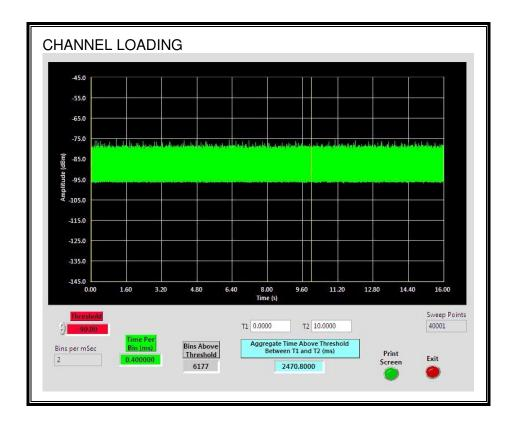
The level of traffic loading on the channel by the EUT is 24.7%
