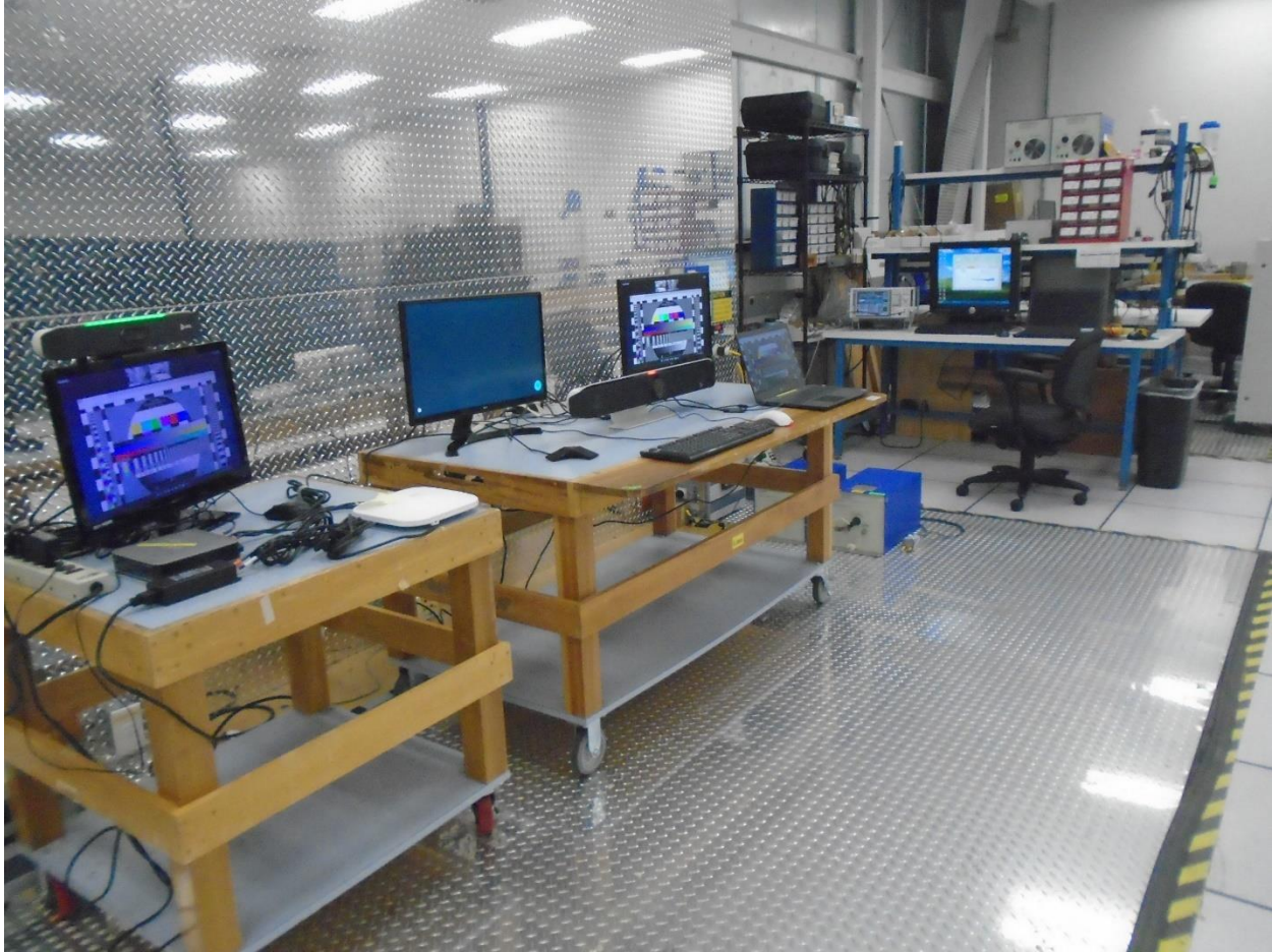
Conducted Emissions Setup
