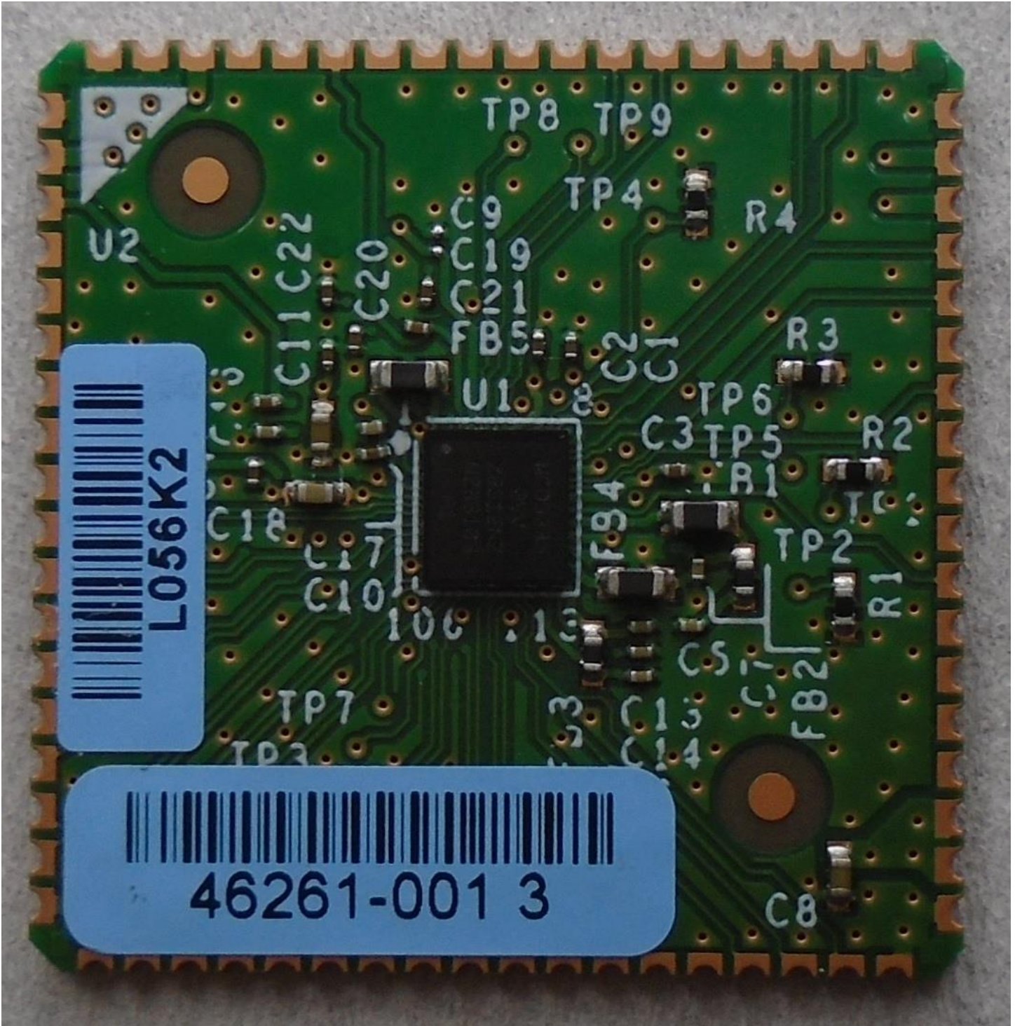
Audio CODEC Carrier PCB Top
