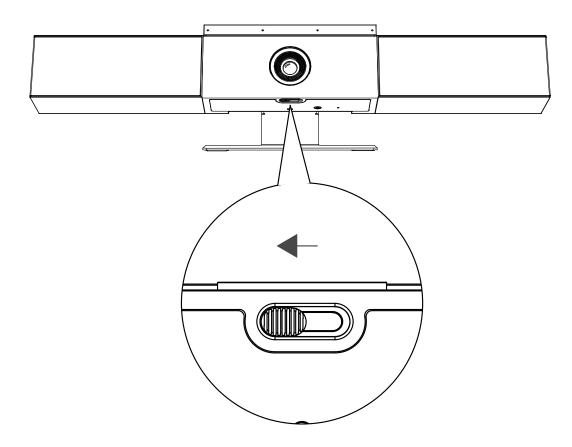
When you slide the lever to the right, the shutter closes and the camera turns off.
