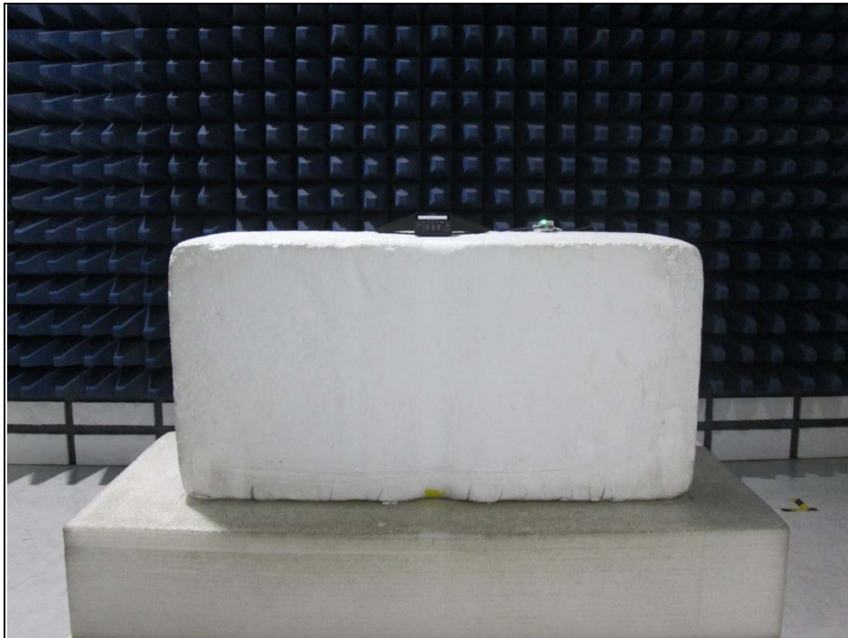
Radiated Emission Test above 1GHz
