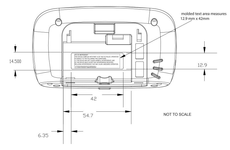
LABEL NUMBER: PD144606C DESCRIPTION: LABEL-MONITOR-VIDEO-PARENT UNIT-FCC LABEL MUST PASS GRACO LABEL SPECIFICATIONS DIMENSIONS: DIE CUT DOES NOT PRINT LOCATION: RAISED MOLD ON VIDEO MONITOR. MOLDED IN TEXT Font: Arial Narrow Molded Letters Text centered in area SPI-A2 Finish
