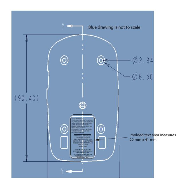
LABEL NUMBER: PD241729A DESCRIPTION: LABEL-MONITOR-BOTTOM HOUSING-2L04-05 LABEL MUST PASS GRACO LABEL SPECIFICATIONS DIMENSIONS:
