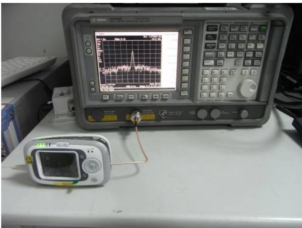
CONDUCTED SPURIOUS EMISSION TEST SETUP
