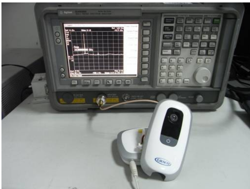
CONDUCTED SPURIOUS EMISSION TEST SETUP
