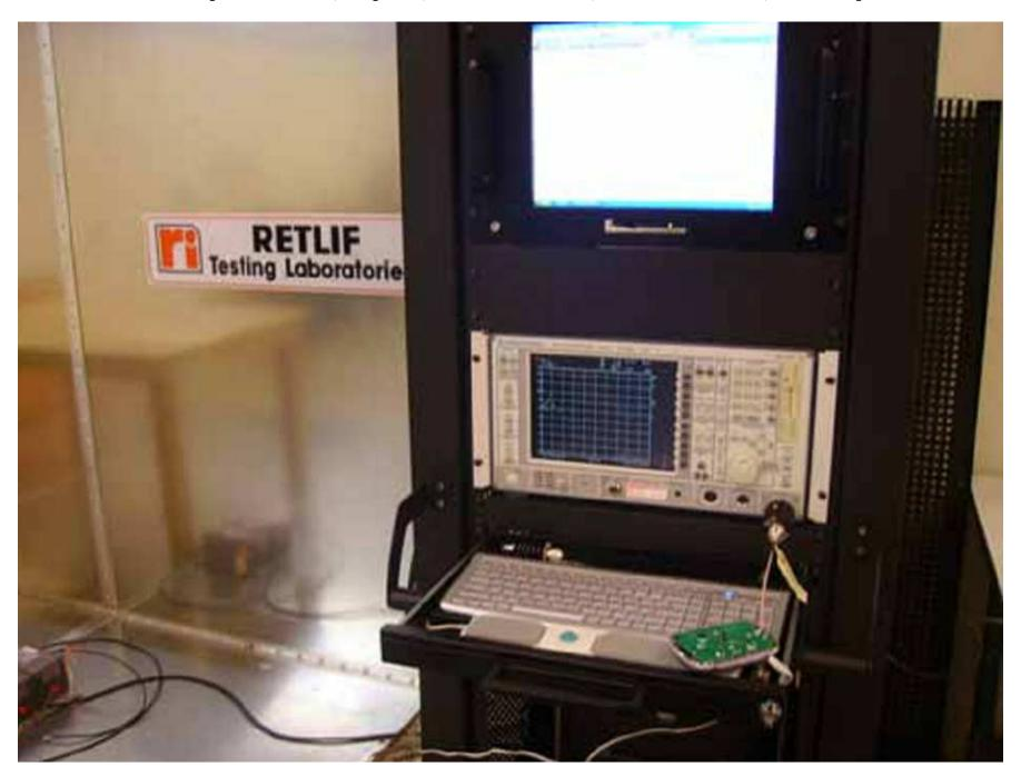
Test Setup – FCC Part 15, Subpart C, Section 15.247 (d), Antenna Port, Conducted Emissions
