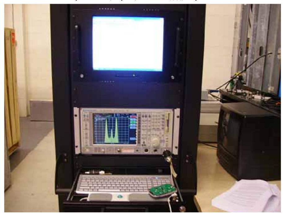
Test Setup – FCC Part 15, Subpart C, Section 15.247 (b) (3), Conducted Emissions, Power Output
