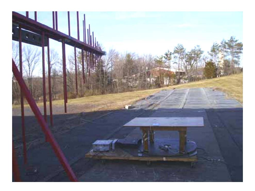
Test Setup – FCC Part 15, Subpart B, Section 15.207 (b), Conducted Emissions, Power Leads, 150kHz – 30MHz
