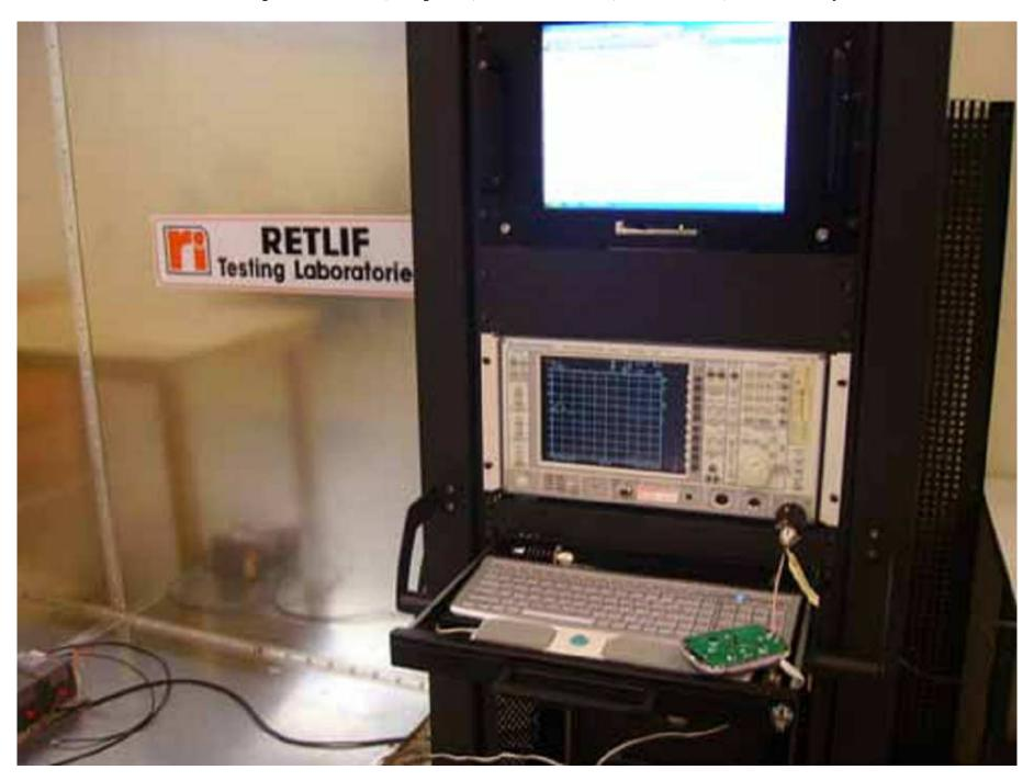
Test Setup – FCC Part 15, Subpart B, Section 15.109 (a), Class B Radiated Emissions 30MHz – 1GHz
