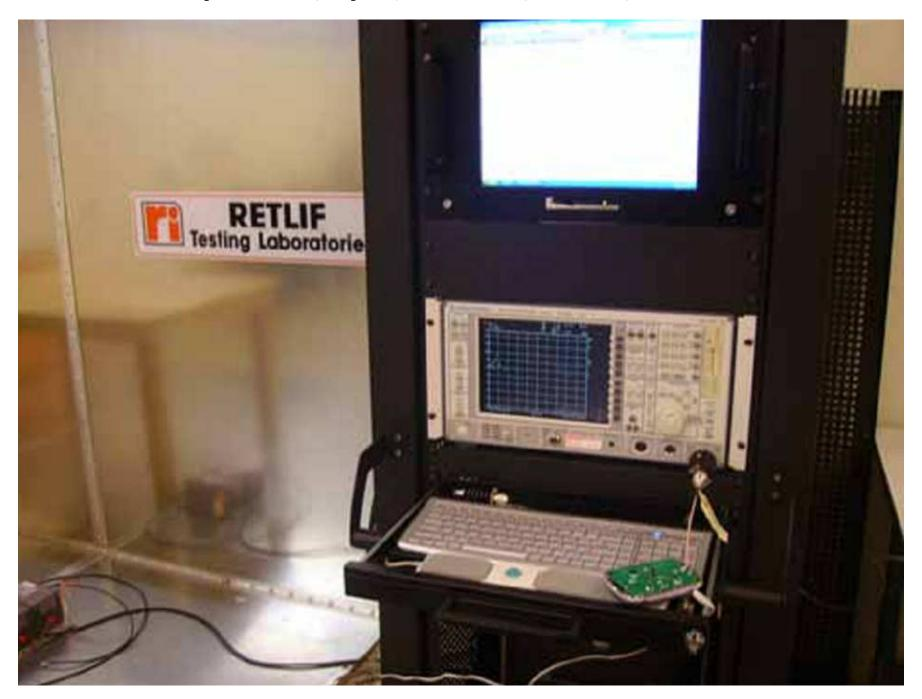
Test Setup – FCC Part 15, Subpart C, Section 15.247 (e), Antenna Port, Power Density
