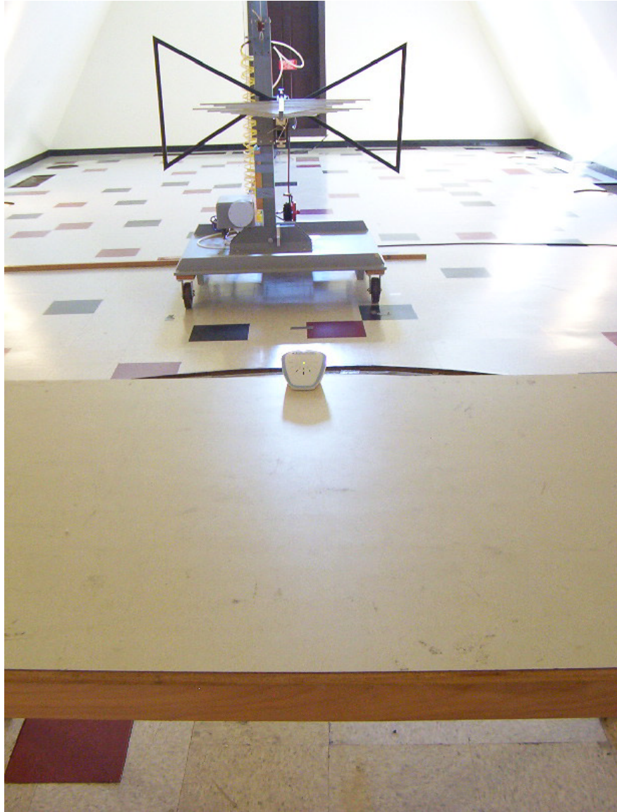
Photo 1: Radiated Emission Test Setup – Front View
