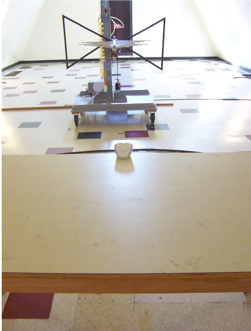
Photo 5: Radiated Emission Test Setup – Front View
