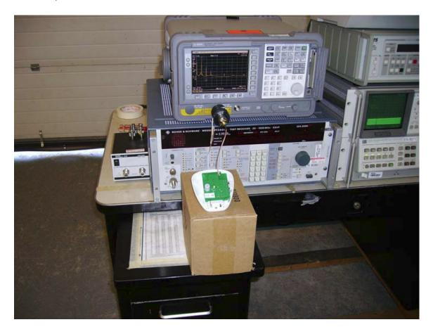
Antenna Port, Power Density FCC Part 15, Subpart C, Section 15.247(e) RSS-210, Section A8.2(b)
