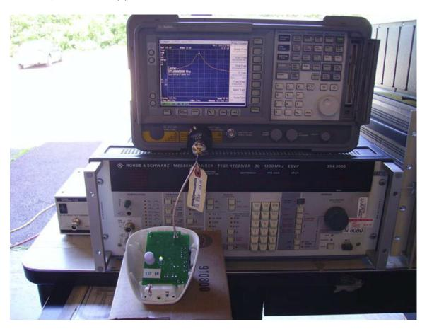
Antenna Port, Conducted Emissions FCC Part 15, Subpart C, Section 15.247(d) RSS-210, Section A8.5
