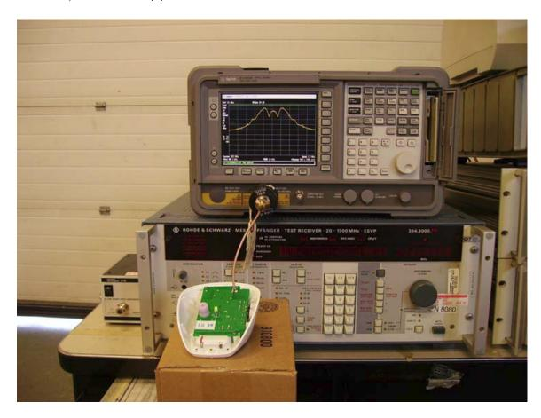
Conducted Emissions, Power Output FCC Part 15, Subpart C, Section 15.247(b)(3) RSS-210, Section A8.4(4)
