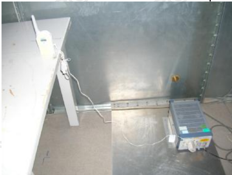
Measurement of Conducted Emission Test Set Up
