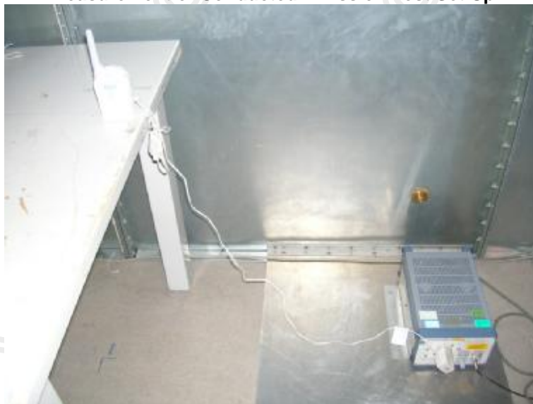
Measurement of Conducted Emission Test Set Up
