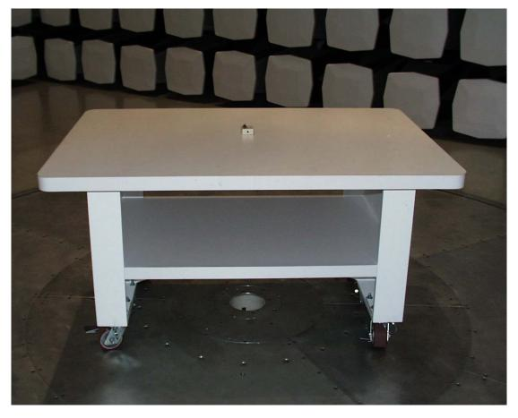
Setup for measurements 30 MHz - 1000 MHz. Measurements were made with the EUT located by itself on an 80 cm high non-conductive table.
