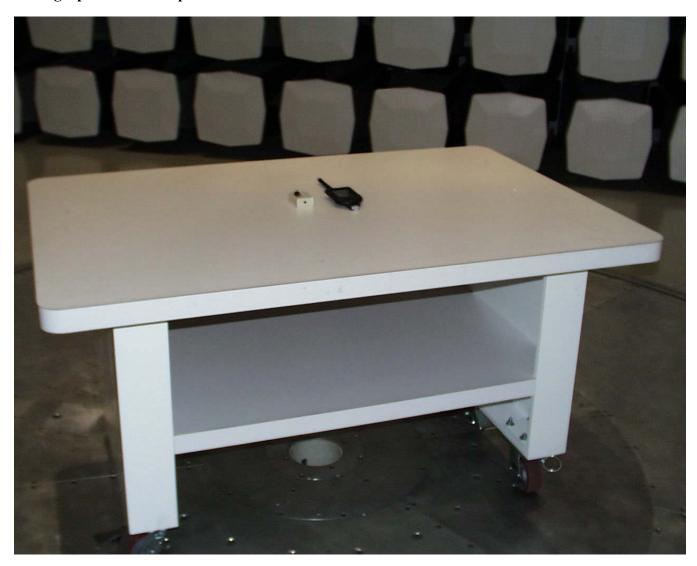
Setup for measurements above 1000 MHz. Measurements were made with the EUT and a Point Six Wireless Transmitter/Receiver (FCC ID: M5ZPTRX) both located on an 80 cm high non-conductive table.
