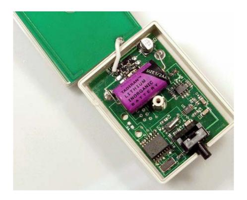
Top View of the Point Six Pressure Transmitter Circuit Board, Model PRES1
