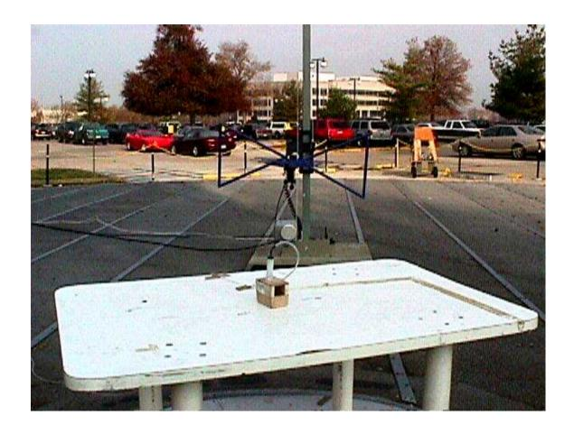
Radiated Test Setup Picture of the Point Six Wireless Sensor
