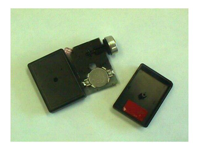
Top View of the Point Six Wireless Sensor Circuit Board.
