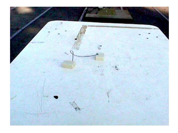
Radiated Test Setup Picture of the Point Six Wireless Analog Sensor
