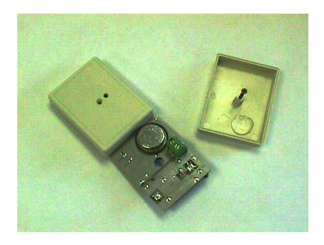
Top View of the Point Six Wireless Analog Sensor Circuit Board
