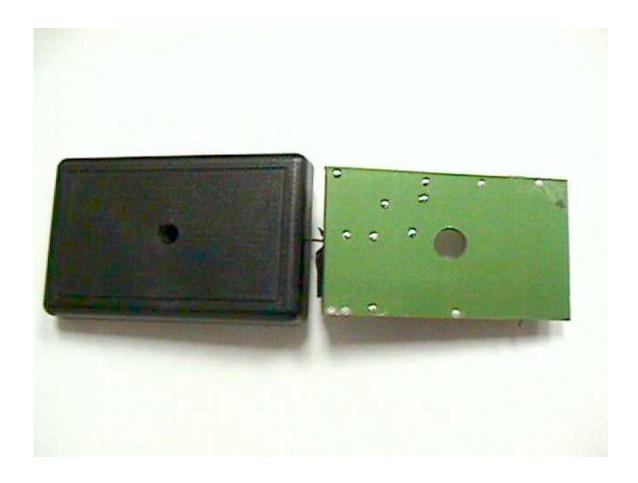
**Bottom View of the Wireless Temperature Sensor Board.**
