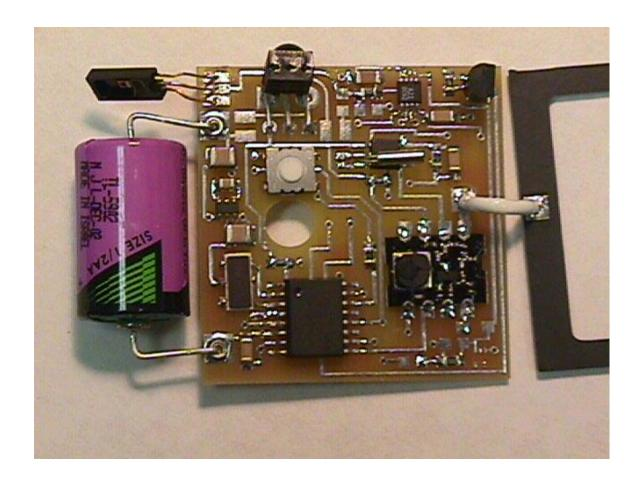
Top View of the Wireless Temp/Humidity Sensor Board.
