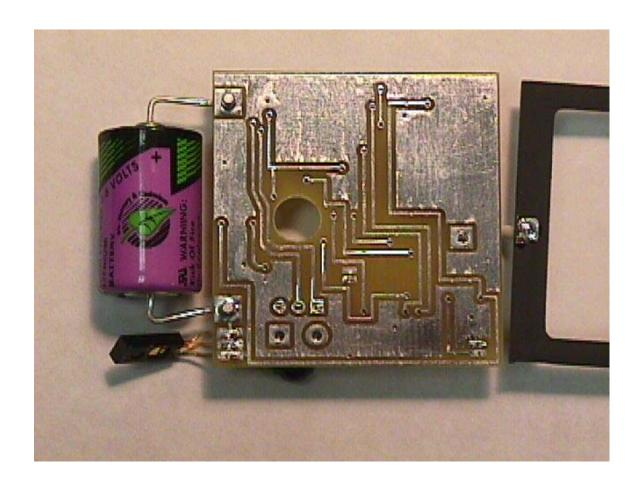
Bottom View of the Wireless Temp/Humidity Sensor Board.
