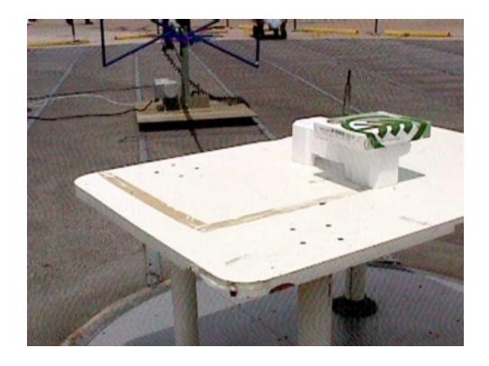
Radiated Test Setup Picture of the Point Six Wireless Temperature probe Transmitter, Model WOW-PRO
