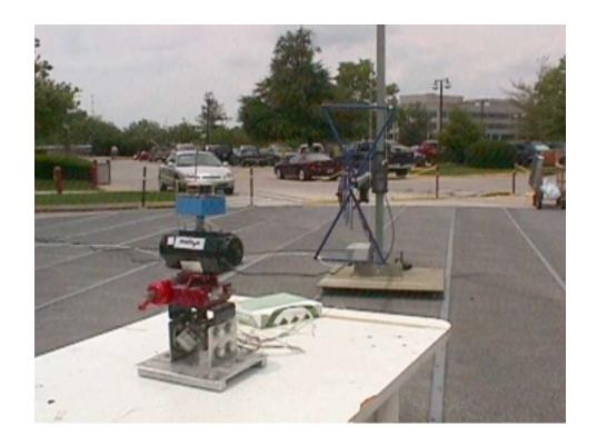
Radiated Test Setup Picture of the Point Six Limit Switch Transmitter, Model LSX-1
