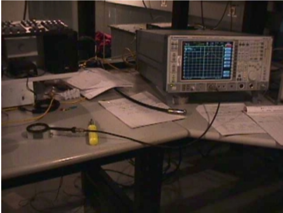
FCC TRANSMITTED BANDWIDTH TEST CONFIGURATION IR PROXIMITY PEOPLE COUNTER 10m/5m SEMIANECHOIC CHAMBER CONTROL ROOM LEXMARK INTERNATIONAL, LEXINGTON KY.
