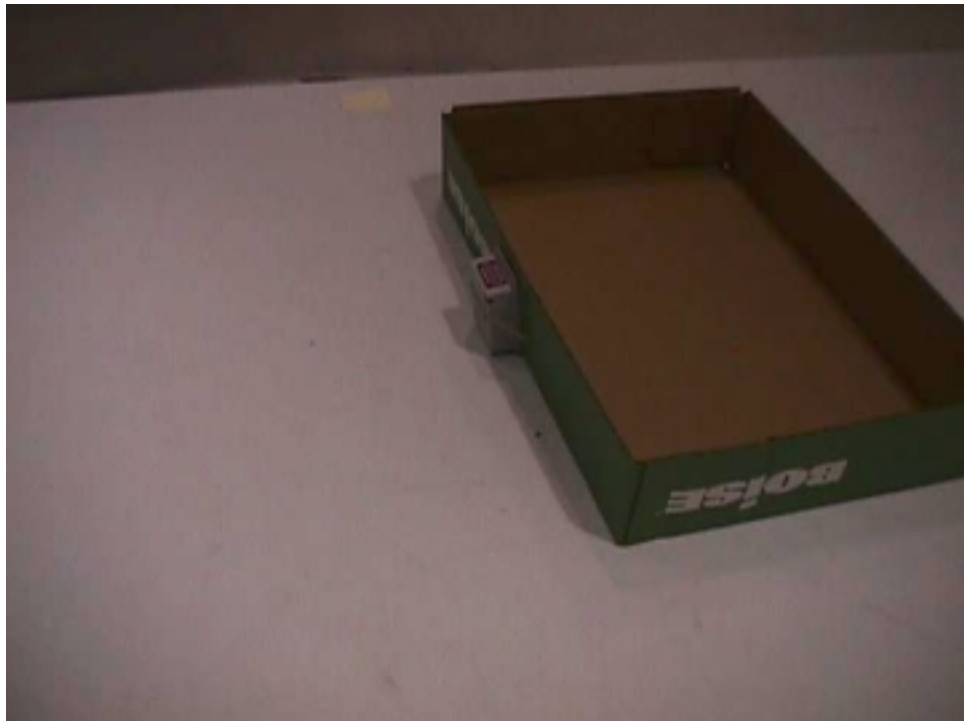
FCC 30-1,000MHz RADIATED EMISSIONS TEST CONFIGURATION IR PROXIMITY PEOPLE COUNTER 5m SEMIANECHOIC CHAMBER LEXMARK INTERNATIONAL, LEXINGTON KY.
