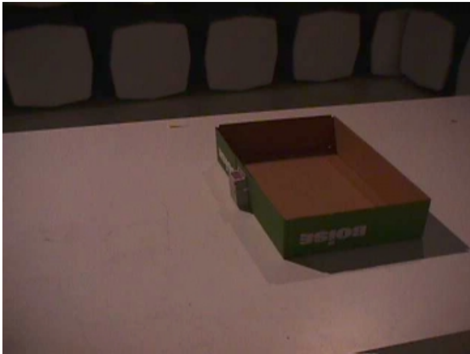
FCC 1,000-4,180MHz RADIATED EMISSIONS TEST CONFIGURATION IR PROXIMITY PEOPLE COUNTER 10m SEMIANECHOIC CHAMBER LEXMARK INTERNATIONAL, LEXINGTON KY.
