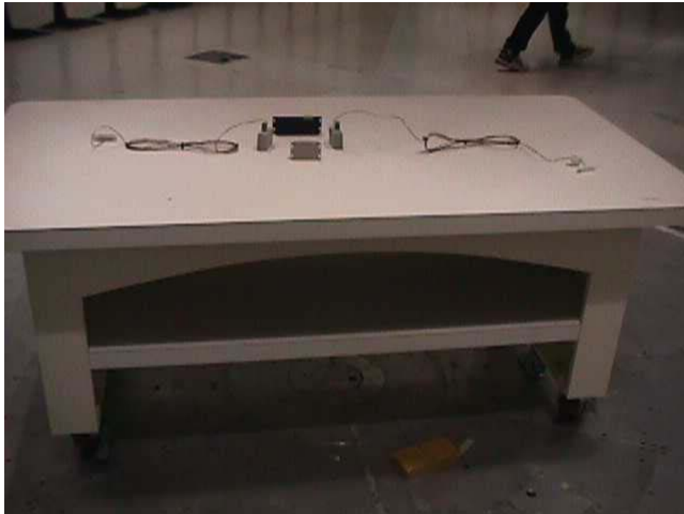
RADIATED TEST CONFIGURATION 30-1000MHz Three Orthogonal Axes
