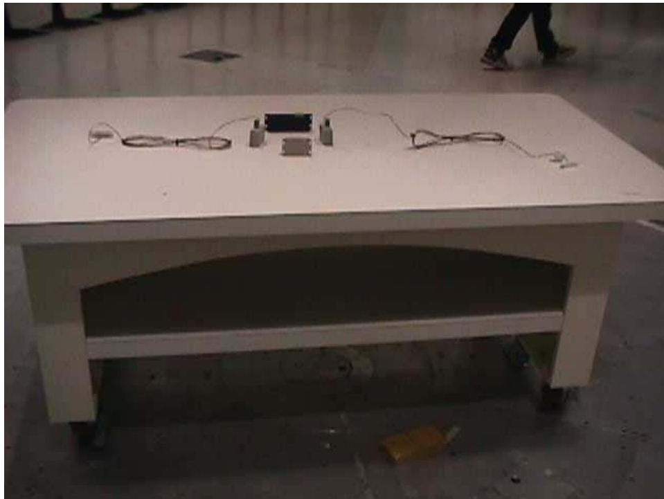
RADIATED TEST CONFIGURATION 30-1000MHz Three Orthogonal Axes
