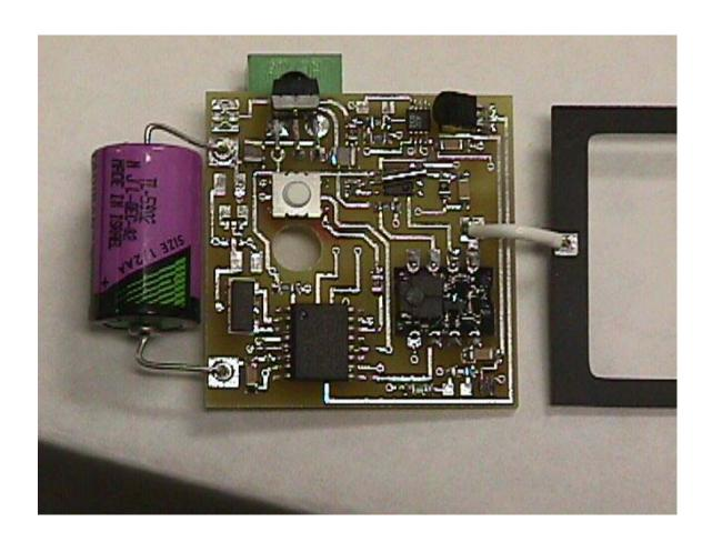
**Top View of the Point Sensor Analog Circuit Board**
