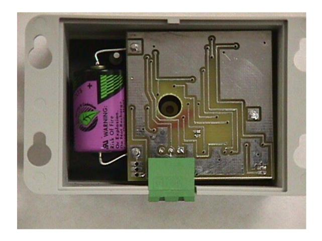
**Bottom View of the Point Sensor Analog Circuit Board**
