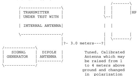
Equipment placed 1 meter above ground on a rotatable platform. The center of the Dipole antenna at the center of the platform and the output of the signal generator adjusted to produce the same meter reading as measured for the fundamental in the radiated emissions test.
