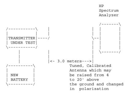
Equipment placed 4' above ground on a rotatable platform.
