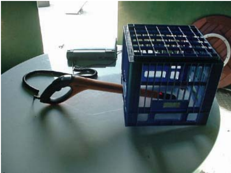
Above 30 MHz test set up – axis 2
