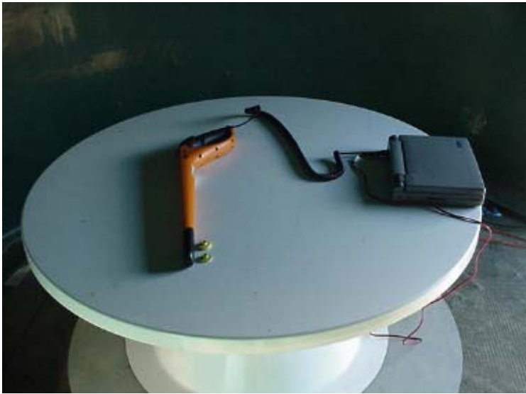
Above 30 MHz test set up – axis 1
