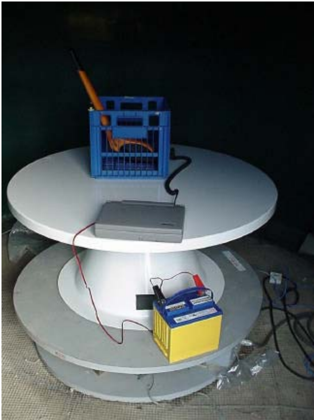
Above 30 MHz test set up – axis 3
