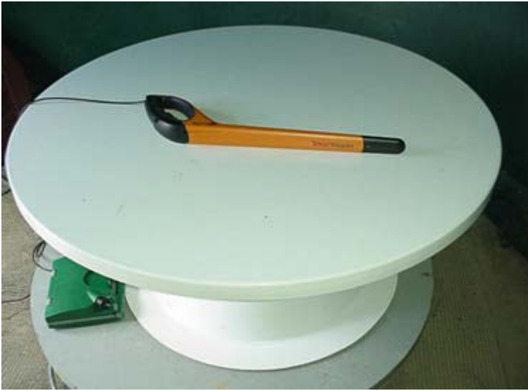
Weigh Scale Powered Test Set Up Laying Flat
