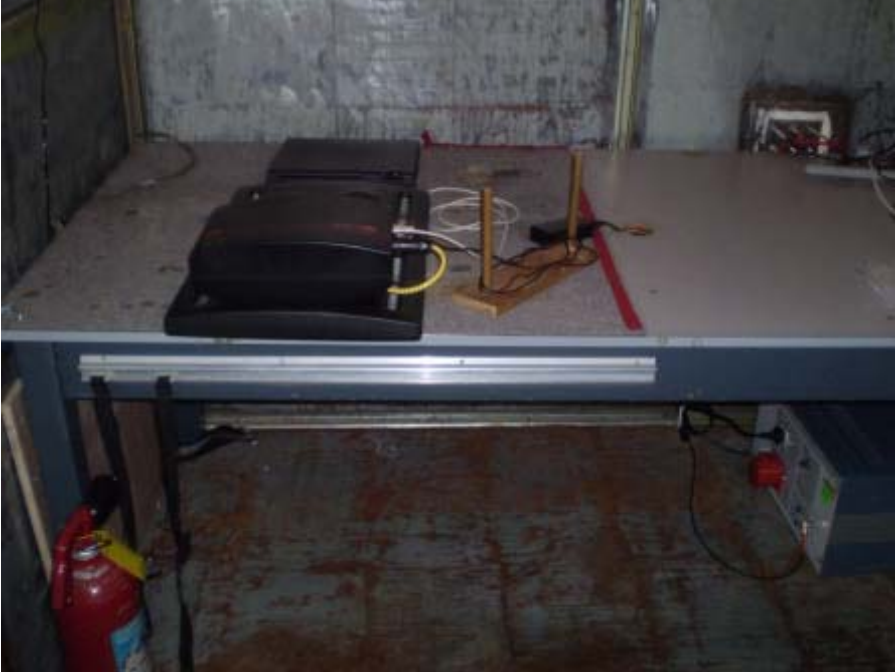
Conducted emissions test set up – Small Panel Antenna
