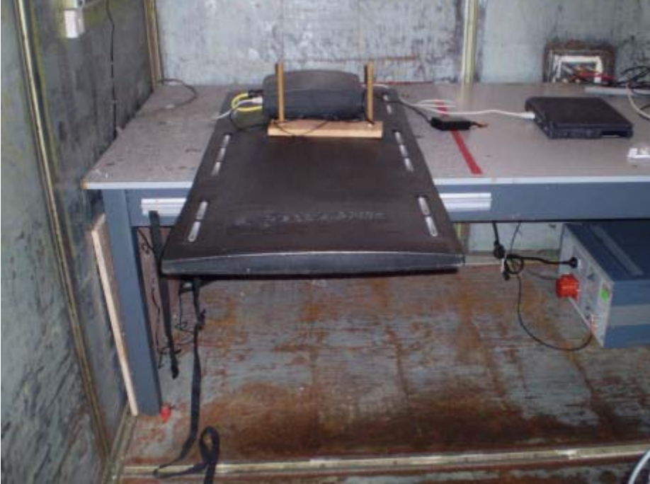
Conducted emissions testing – Large Panel Antenna
