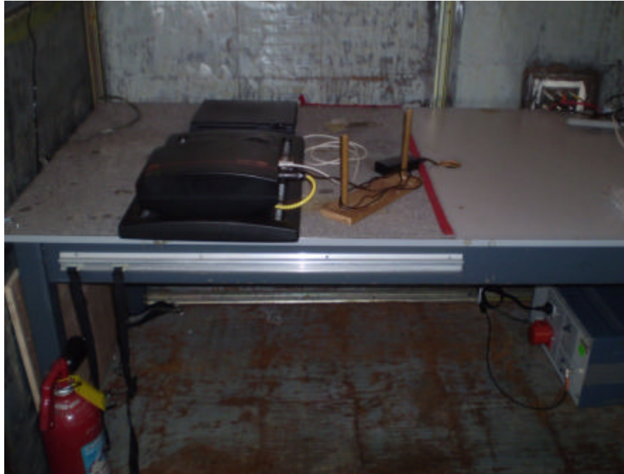
Conducted emissions test set up – Small Panel Antenna
