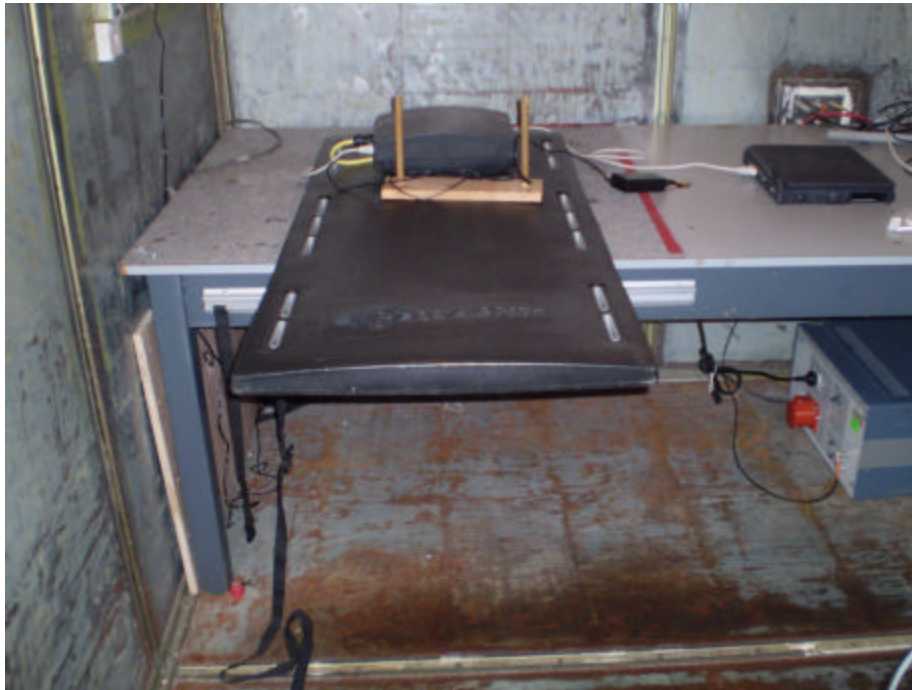
Conducted emissions testing – Large Panel Antenna
