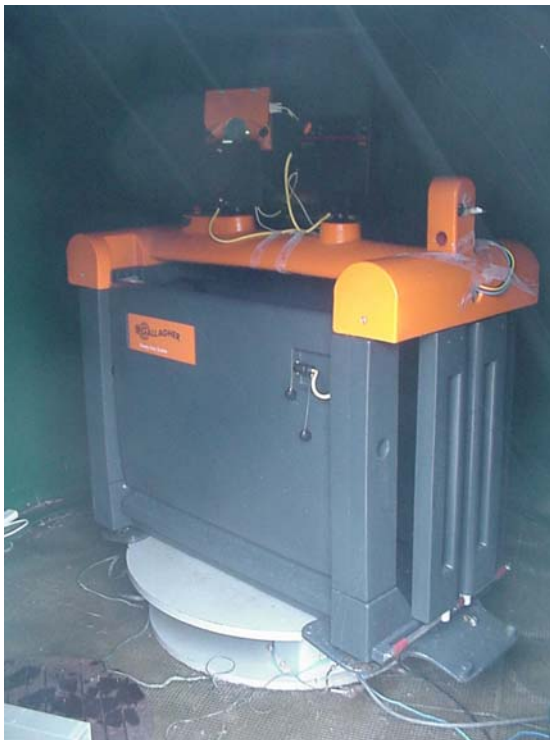
Radiated emissions test set up above 30 MHz
