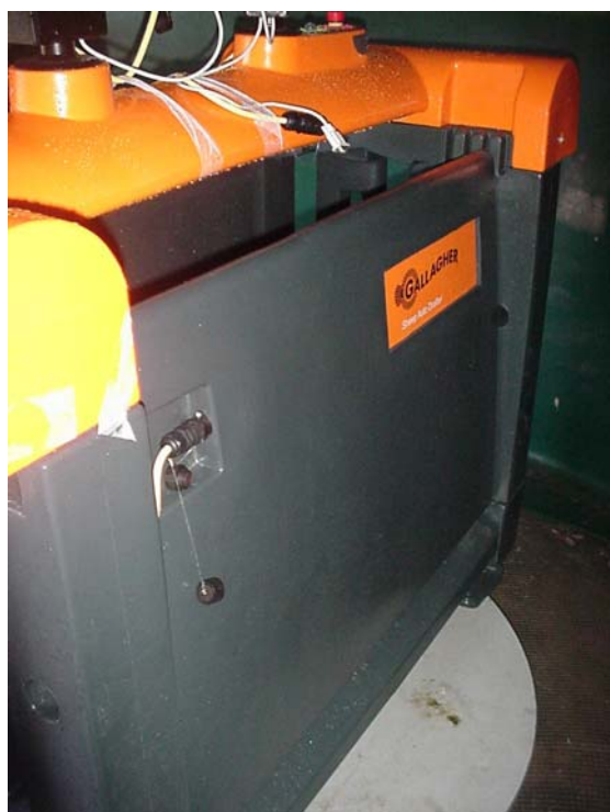
Radiated emissions test set up above 30 MHz
