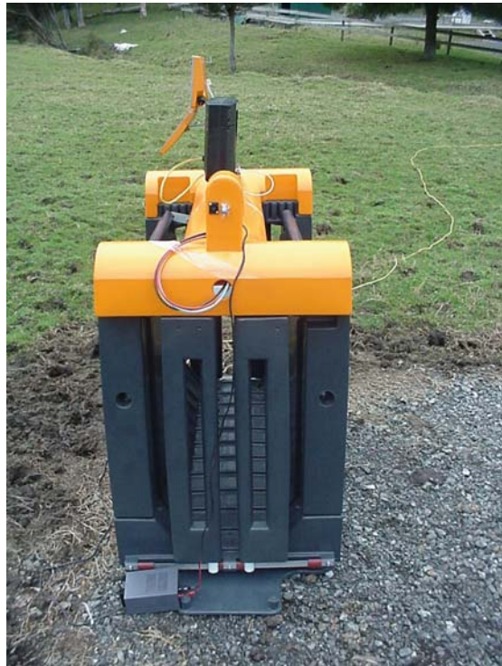
Radiated emissions test set up above 30 MHz
