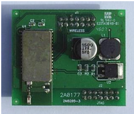
Bluetooth Module PCB - Component Side
