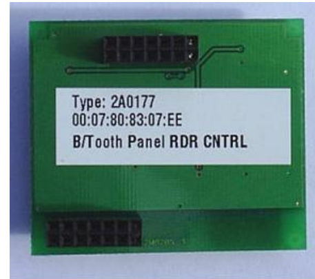
Bluetooth Module PCB - Solder Side
