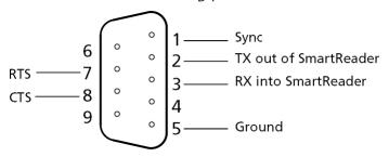
This cable in not supplied by Gallagher - you are expected to have a custom cable made to suit the individual installation.
