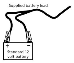
Connect the **Red** clip to the **Positive** terminal Connect the **Black** clip to the **Negative** terminal.
