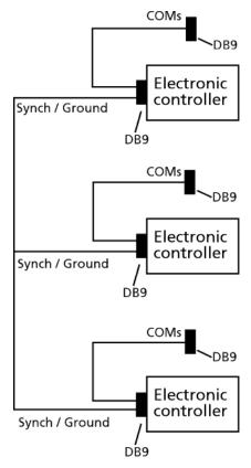
The extra COM connectors enable you to alter the settings of each SmartReader.
