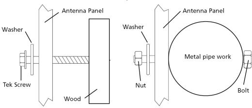
4. Using the **defined mounting holes**, mount the Antenna Panel on the **outside** of the animal handler so that the middle of the Antenna Panel matches the average height.
