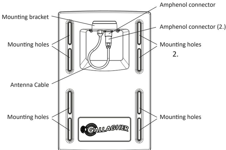
3. Connect the extension cable to the Amphenol connector and tighten, then connect the other end of the extension cable to the Antenna connector on the base of the TWR-5.
