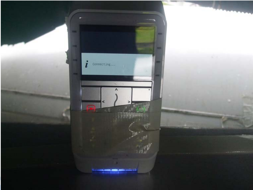
Ancillaries placed at a distance from product under test during radiated emissions test
