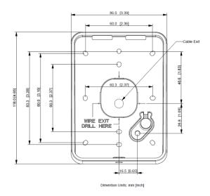
4. Drill pilot holes for the four corner fixing holes and the tamper tab. Secure the bezel to the mounting surface using the four corner fixing screws provided. Secure the tamper tab (located in the bezel) to the mounting surface using the remaining fixing screw provided. It is important the four corner fixing screws are used to ensure the terminal is flush with and tight against the mounting surface.
