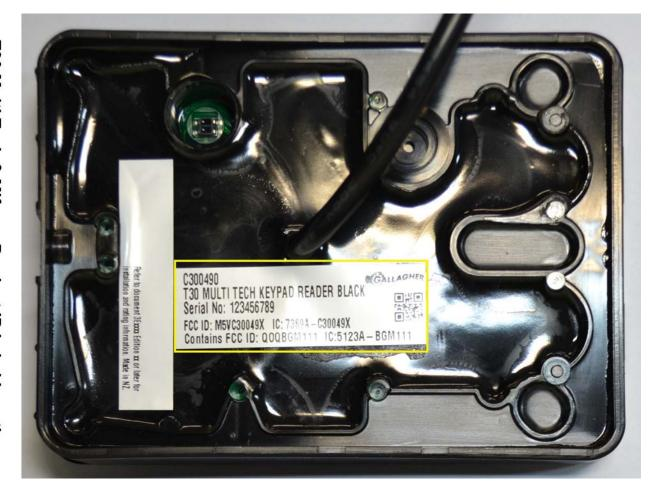
Product is sold with mounting bracket which is required to be removed exposing label prior to install. This meets CFR 47.2.925(d)(2).
