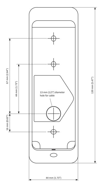
**IMPORTANT** This picture is not to scale, therefore use the measurements provided.
