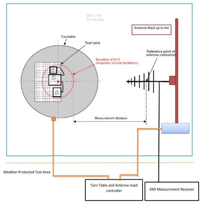
Below 30 MHz: Loop Antenna; Measurement distance: 10 m
