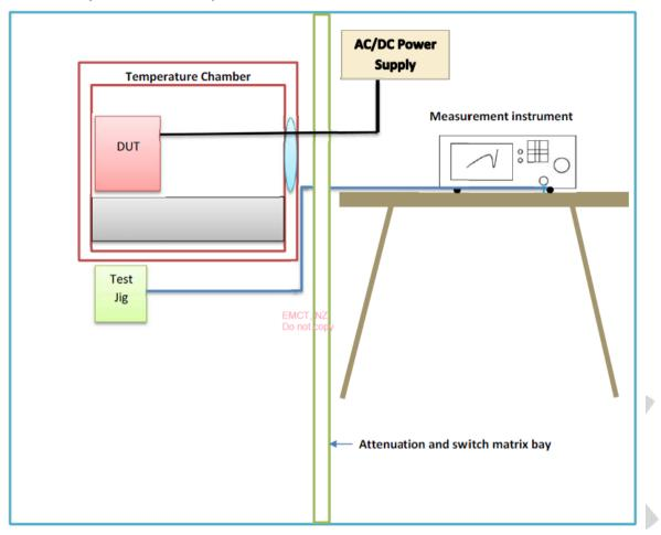
Following test instruments were used to carry out this test:
